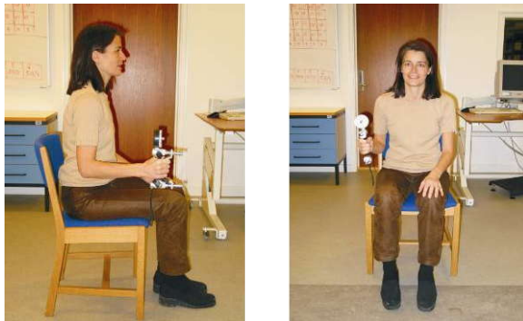
Figure 5. Set-up for measurement of maximal hand-grip strength.
