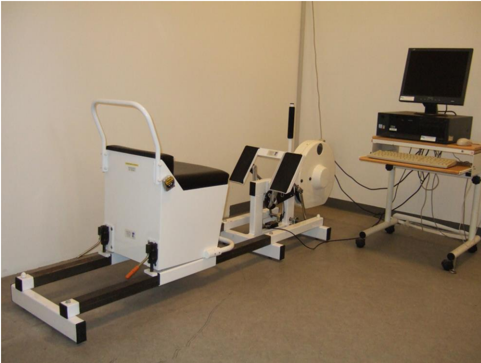
Picture 5. Nottingham Leg Extensor Power Rig
