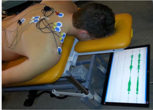
Figure 5. Picture of experimental setup and electrode placement at clavicular, descending, transverse and ascending compartments of the trapezius muscle. Reference electrodes (REF) was placed at the acromion and C7.
