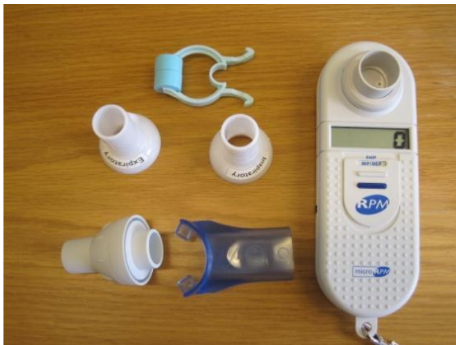
Figure 5: Micro RPM used for measurement of respiratory muscle strength.
