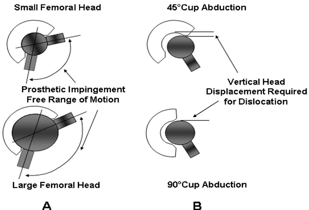
Figure 12. Impingement free movement and VHDD with large heads. (39)
