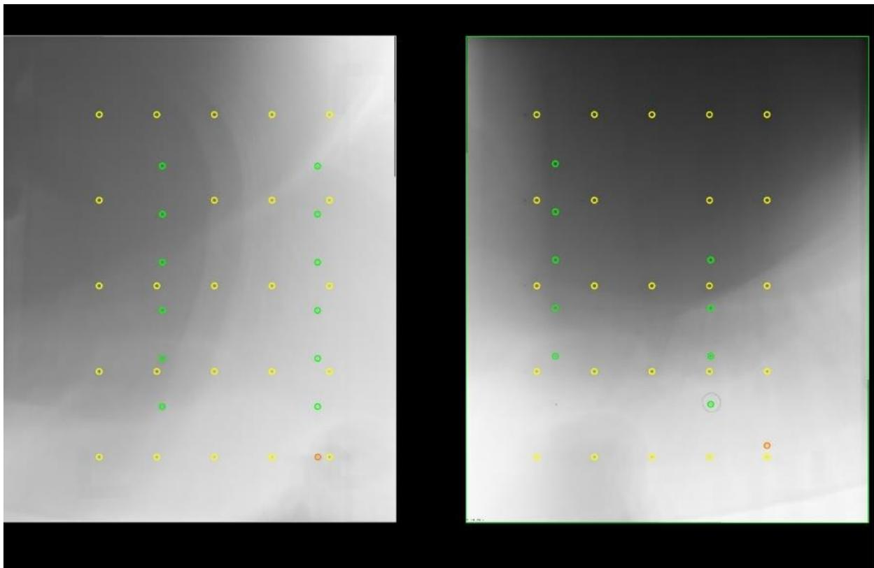
*Figure 16. Calibration image for dynamic RSA analysis. The moving implant appears as a blur, and the calibration markers are clearly visible.*
