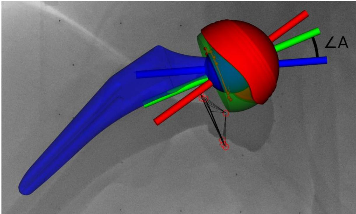
Figure 19. Y-axis of the shell, liner end neck coordinate systems with the liner/neck angle ( $A$ ) (5).
