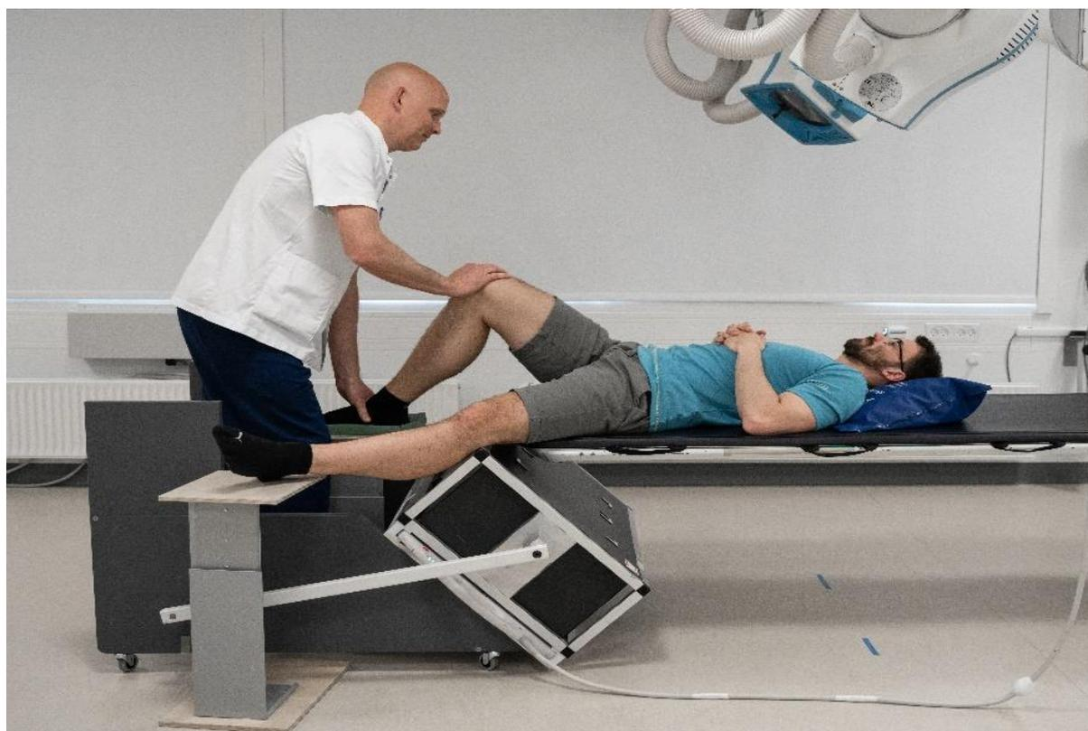
*Figure 15. The dynamic RSA setup. X-ray tubes and calibration box were angled 45° for better view of implants throughout the recording (6).*
