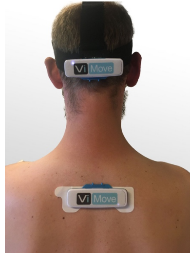
Figure 9 Placement of the ViMove sensors. One was placed on a hairband and another over T3 on the skin.
