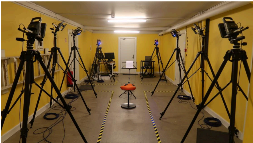
Figure 16 The Vicon motion capture system used in the attic at Bispebjerg Hospital.
